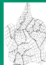
Finite element schematization of the Vyatka River basin
