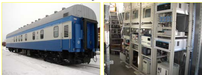
Fig.7. Carriage – observatory. The complex equipped with measuring instruments manufactured by the leading world manufacturers provides round-the-clock all-the-year-round continuous measurements of all basic gaseous species: ozone, nitrogen monoxide and dioxide, carbon monoxide and dioxide, methane, sum of non-methane hydrocarbons, sulfur dioxide and ammonia.
